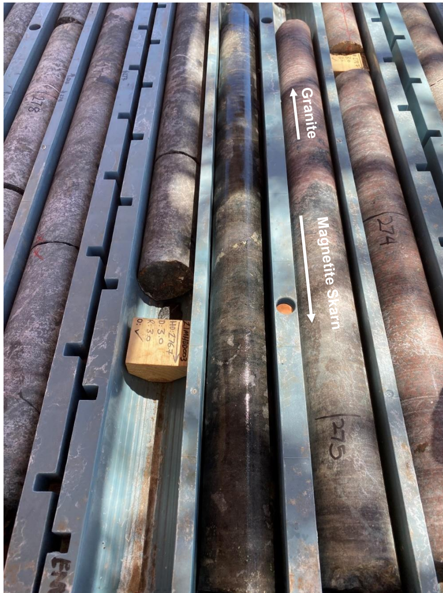
Photo 3: 21MHDD003 (273.5– 283.5m) – massive magnetite skarn with disseminated scheelite and molybdenite (metallic silver) mineralisation and bands of chalcopyrite (yellow).
