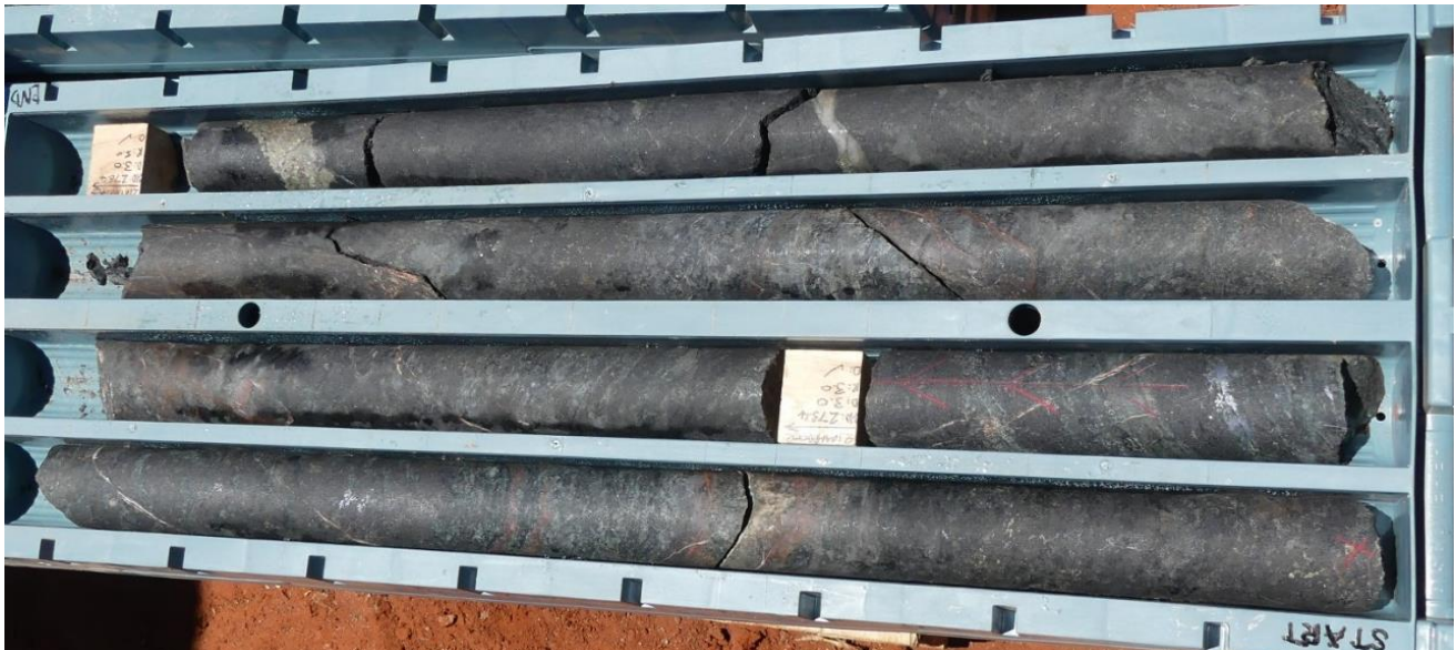
Photo 2: 21MHDD002 (272.2 – 275.7m) – massive magnetite skarn with disseminated scheelite and molybdenite (metallic silver) mineralisation and bands of chalcopyrite (yellow).
