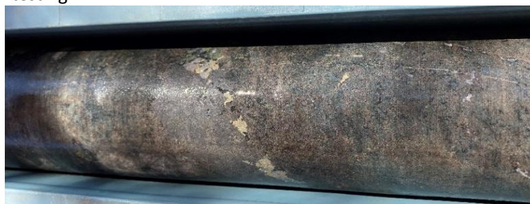
Photo 1: 21MHDD03 – 276m; scheelite-molybdenite-chalcopyrite disseminated mineralisation within magnetite skarn
