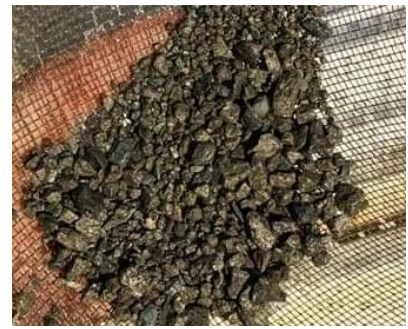
Figure 12: RC chips from KMRC022 84-85m showing massive sulphide mineralisation comprised of pyrrhotite-pyrite (bronze-yellow) and chalcopyrite (golden-yellow). This metre assayed 7.4% Cu, 132g/t Ag, 6.2 g/t Au.
