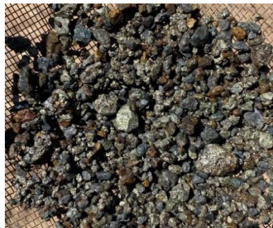
Figure 11: RC chips from KMRC039 18-19m showing supergene mineralisation comprised of chalcocite (dark grey) mixed with pyrite, chalcopyrite and gossanous iron oxides. This metre assayed 12.5% Cu, 129g/t Ag, 1.9 g/t Au, 0.05% Co.
