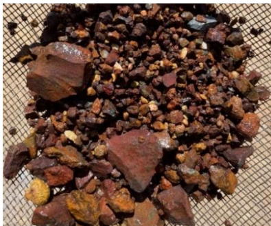
Figure 10: RC chips from KMRC047 4-5m showing oxide mineralisation comprised of gossanous iron oxides (red-brown) and secondary copper carbonates (green). This metre assayed 3.25% Cu, 19.6g/t Ag, 1.9 g/t Au.
