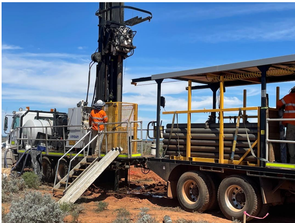
Figure 2 – Sonic core drilling rig on Blackbush deposit, Sapphire Uranium Project
