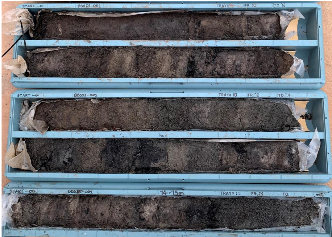
Figure 3 - Sonic core hole BBS21-001 from 70 to 75 metres depth at Alligator's Whyalla core shed prior to geological logging and sampling
