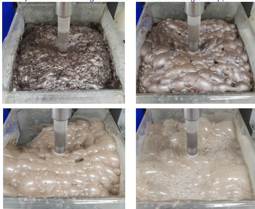
Photos 1 to 4: Webbs Consol rougher flotation concentration stages 1 to 4 (Drill hole WCS007 1,2 )
