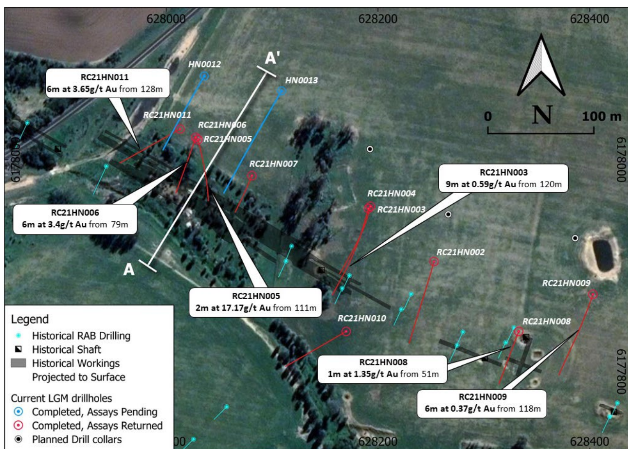
Figure 3. Plan of Harden Gold Mine Prospect drill collars and hole traces
