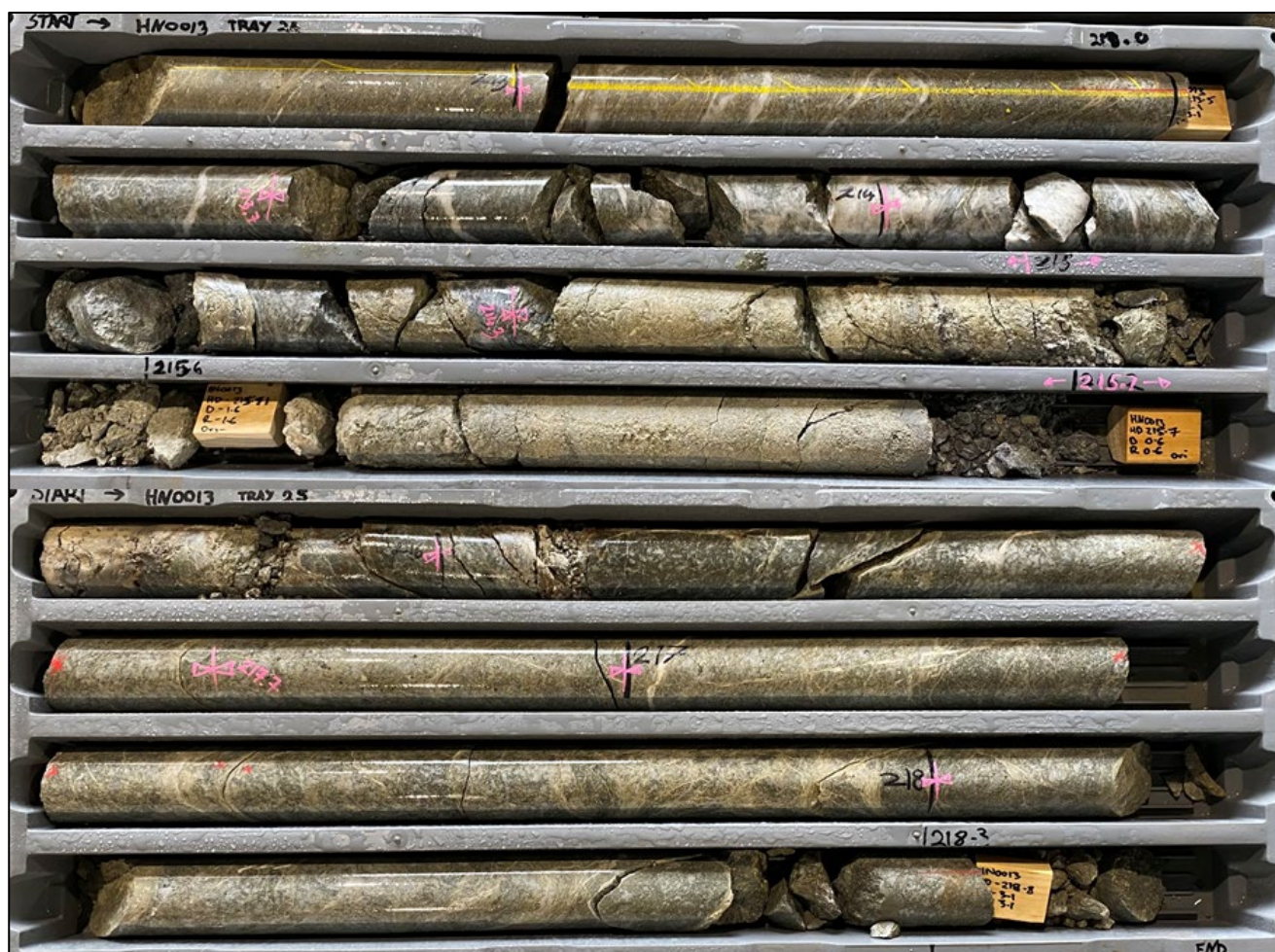
Figure 4. HN0013 drill core; part of the interval from 209m to 224m (down-hole) showing quartz veining and unhealed fault within intensely sheared quartz-sericite-pyrite altered granodiorite containing occasional coarse arsenopyrite and variably rich fine to very fine sulphides (pyrite-arsenopyrite +/- galena-sphalerite) in quartz veining.
