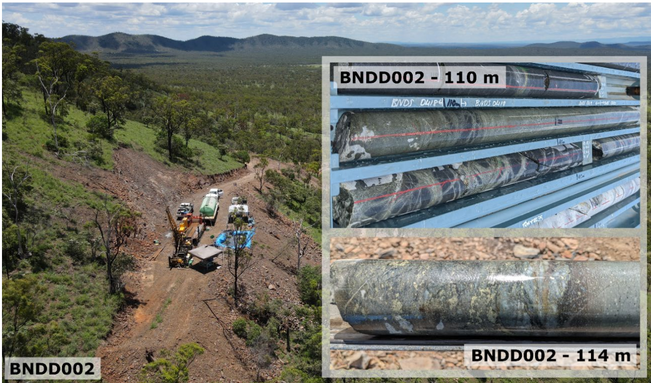
Figure 9. Isens drill rig set up on the pad drilling NW with examples of mineralised lodes intersected downhole
