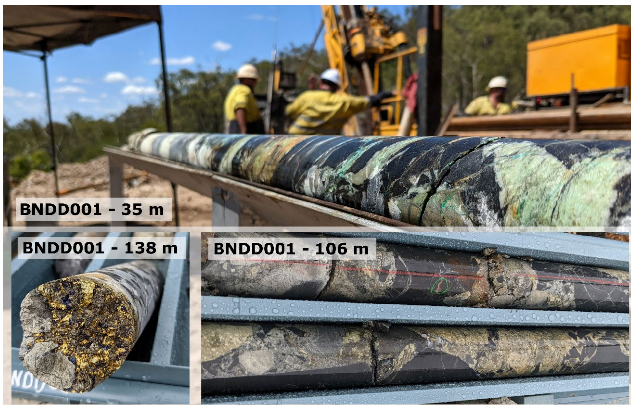
Figure 6. Quorn BNDD001 mineralised zones intersected downhole showing breccia style mineralisation
