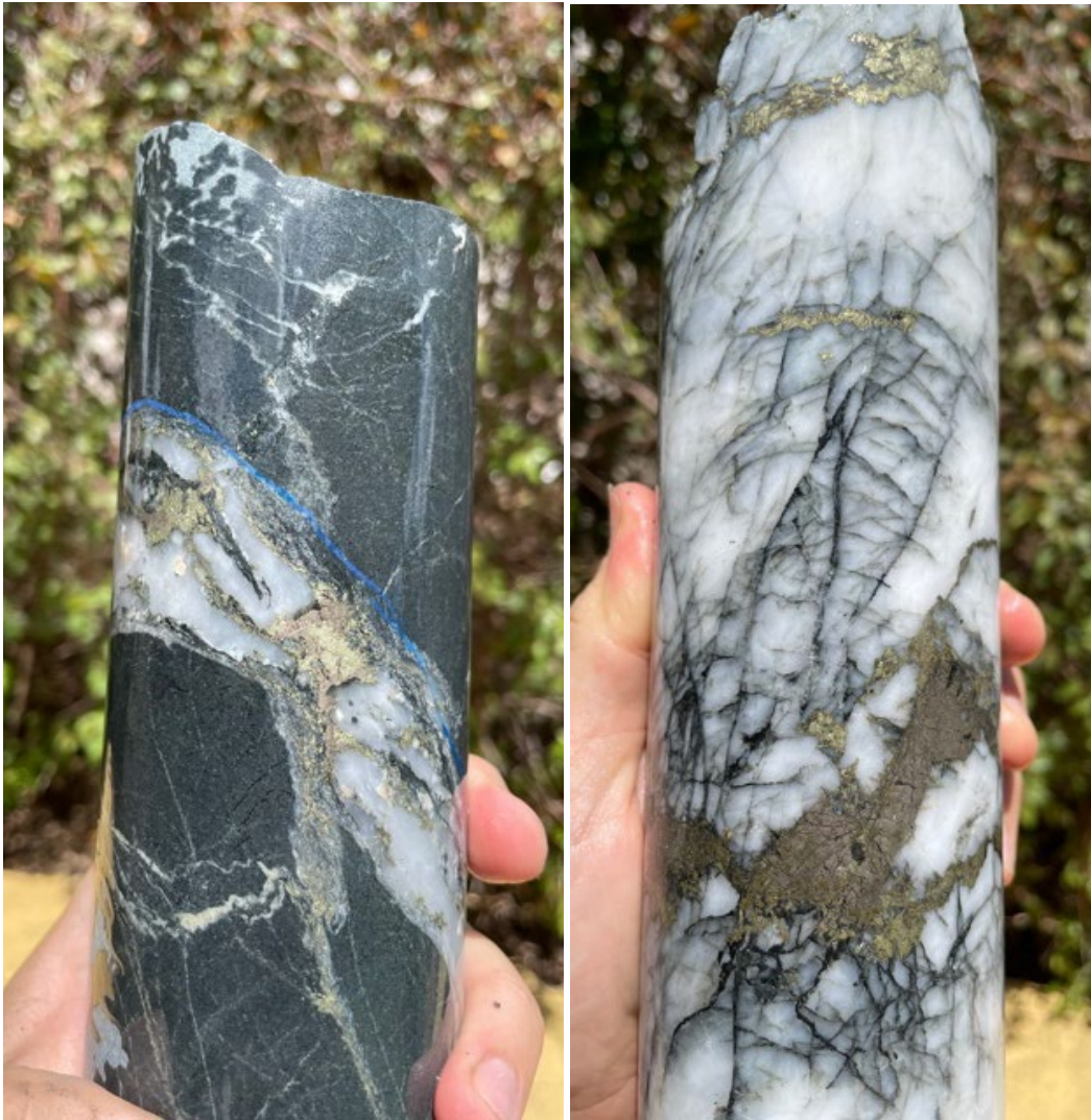
Figure 8. BTDD004 (364.9m, left). Quartz-pyrite-chalcopyrite vein. BTDD004 (376.8m, right). Buck quartz-chalcopyrite-pyrite-pyrrhotite fracture infill vein.
