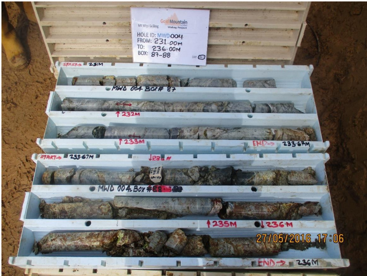
Figure 6. Skarn intersected in MWD004 cut by numerous quartz veins which are high in iron oxides (possibly after sulphides in places)
