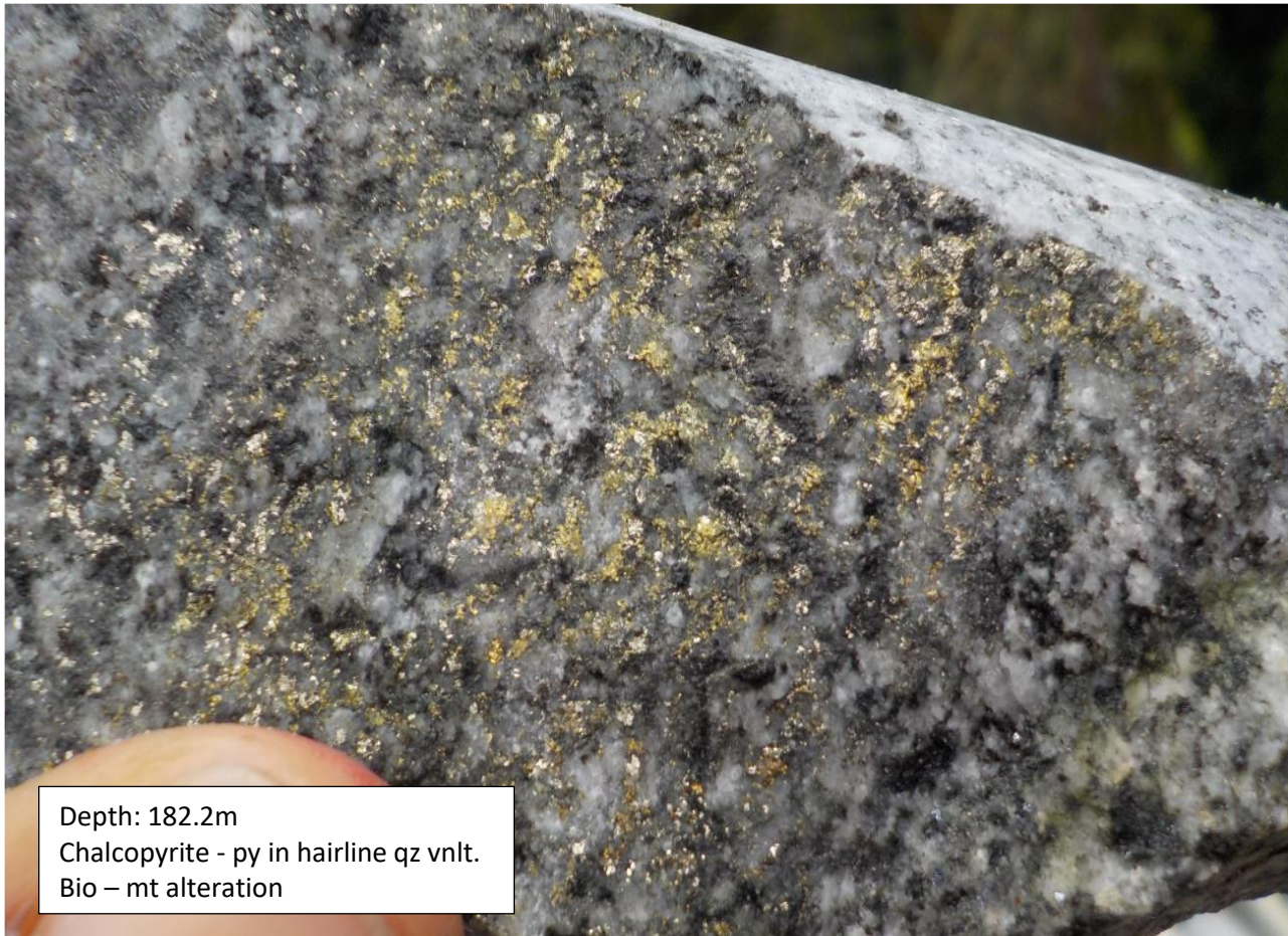
Figure 4. MWD003, Pyrite + Cpy to 1% coating- fracture surfaces in MWD003
