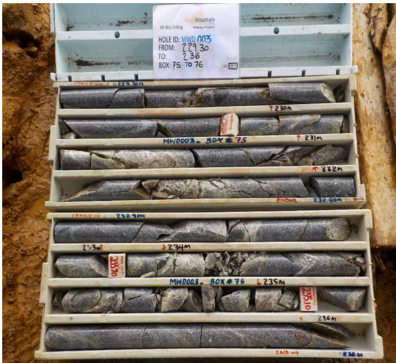
Figure 3. MWD003 from 229.30m to 236m, strongly fractured micro-diorite cut by quartz veins and exhibiting localised bleaching
