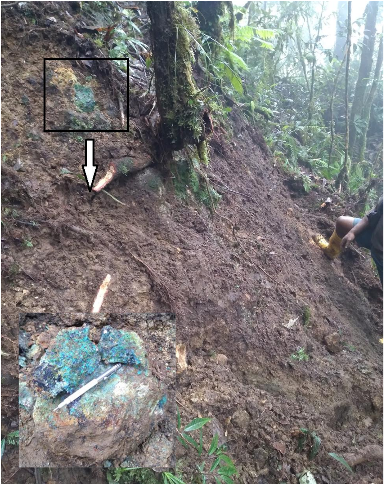
Figure 8. Kandum Prospect, showing malachite rich boulders in the exposed face, this section was channel sampled (Sample numbers MWR139 to MWR144) and averaged 0.20% Cu and 0.1g/t Au over a 60m interval
