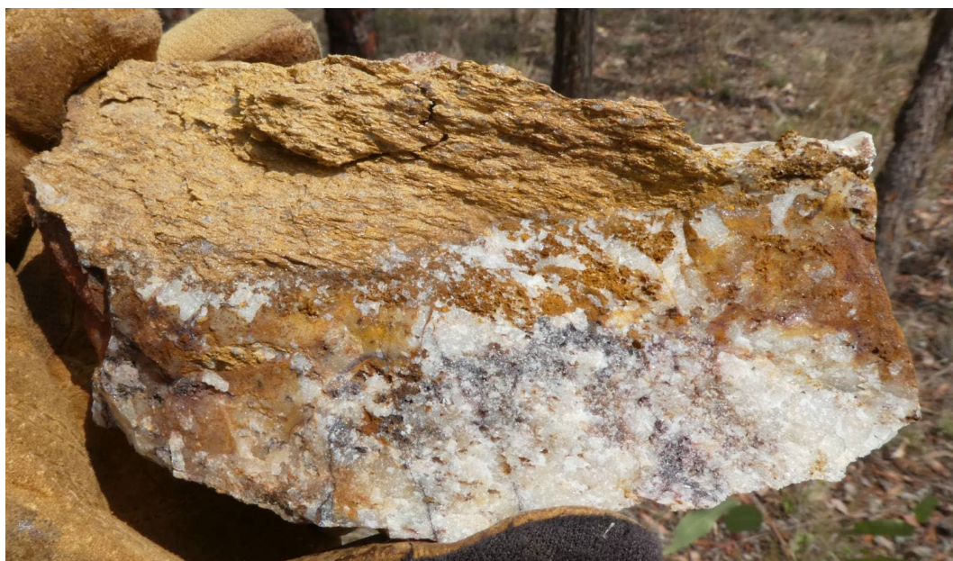
Figure 4. Granular quartz vein with boxworks after pyrite from the Origin prospect. Schistose wall-rock is tonalite with intense quartz-sericite-pyrite alteration.
