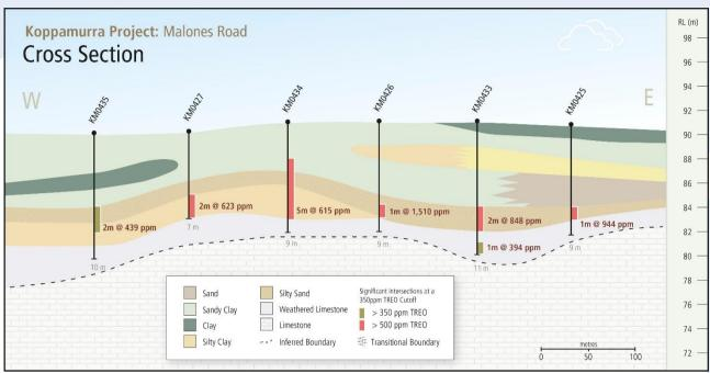
Figure 3 – Cross Section B – Malones Road
