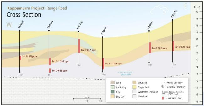
Figure 2 – Cross Section A – Range Road
