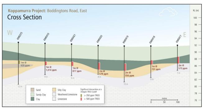
Figure 4 – Cross Section C – Boddingtons Road, East
