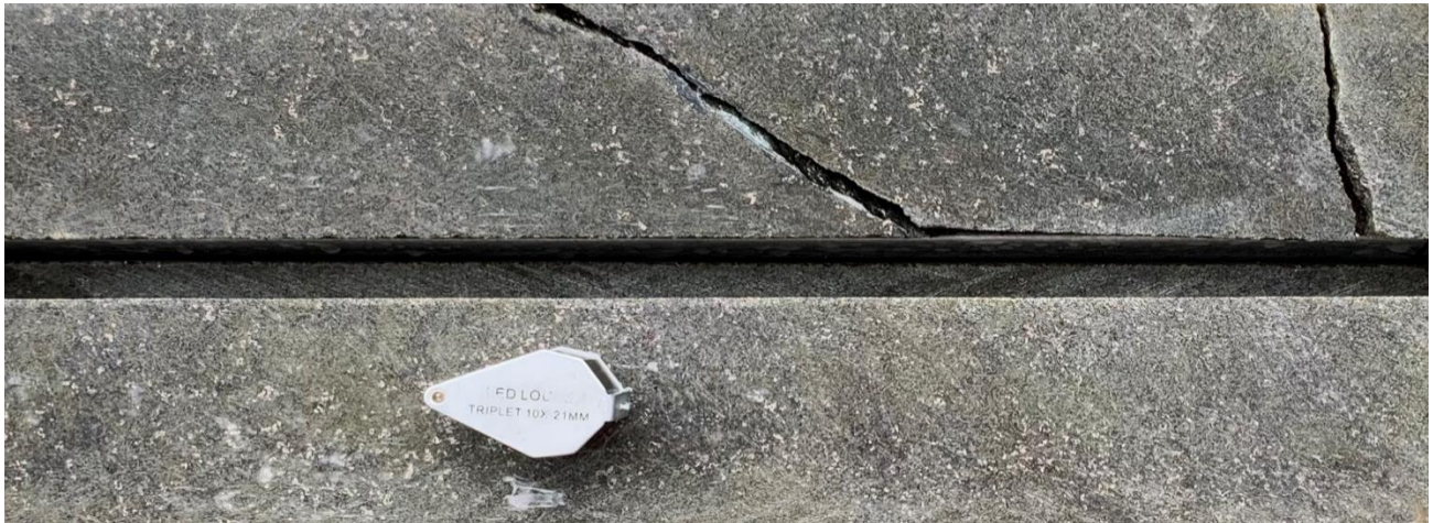
Figure 4 - Disseminated Sulphides over the 148 to 161m interval. The top image has disseminated sulphides throughout. The bottom image is zoomed in to a portion of the core to make them more visible.
