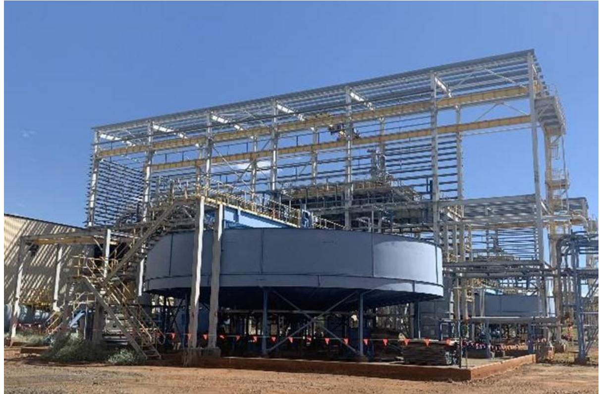
Tailings Filtration system including filter press (background) and thickener (foreground) that PNX is assessing for use at the Fountain Head project. The equipment would be transported and reconstructed at Fountain Head
