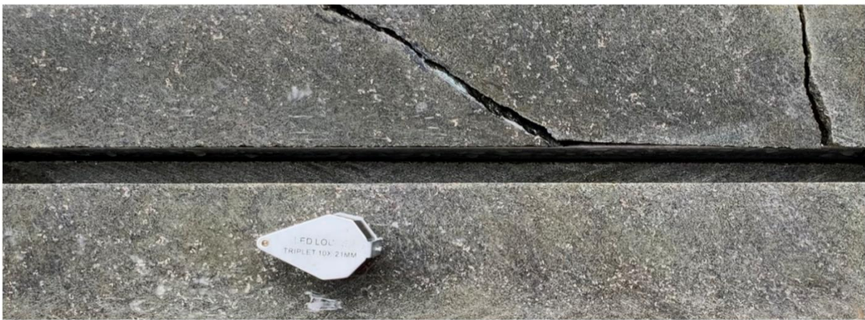
Figure 2 – Zoomed in image of core showing disseminated character of sulphides throughout 148 to 161m interval.
