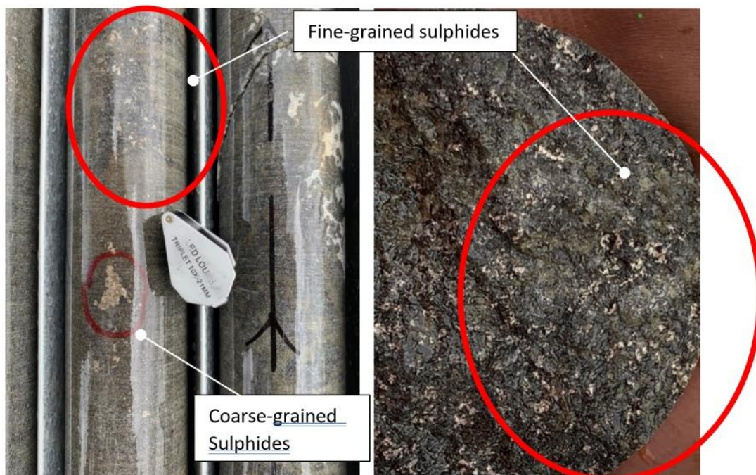
Figure 3 – Showing coarser blebby sulphides from 130.2 and 132m on left and disseminated sulphides on broken face of core on the right.
