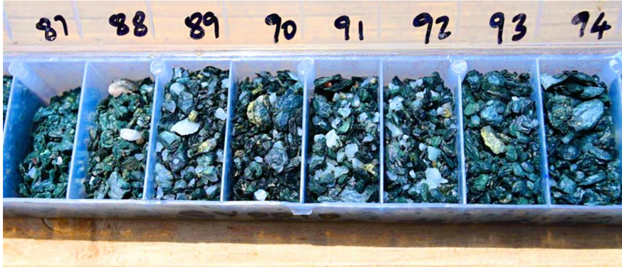
Figure 1: A small section of Copper mineralisation (chalcopyrite) intersected in RC chips from hole CV0010, 87 to 94m shown of a broader mineralised interval of 84 to 96m
