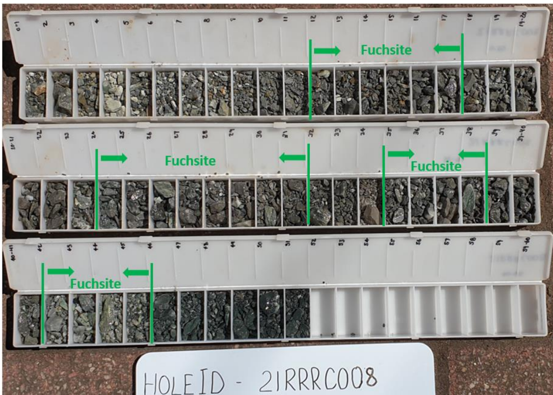
Photo Plate 1 –Fuchsite (chromium rich muscovite) alteration in 21RRRC008
