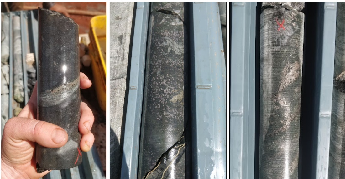
Figure 1: WARDH0065 a. Quartz+/-carbonate +/-pyrite vein in chlorite altered sedimentary rocks; b. Garnet+pyroxene+chlorite skarn alteration (~58m); c. semi-massive sulfides (pyrrhotite dominant) associated with skarn alteration of sedimentary rocks (~61m)
