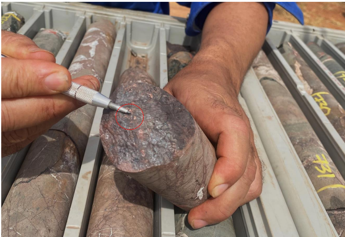
Figure 2: Slickensided parting KNRDD002 with fine native copper indicated at approximately 732.5m down-hole.
