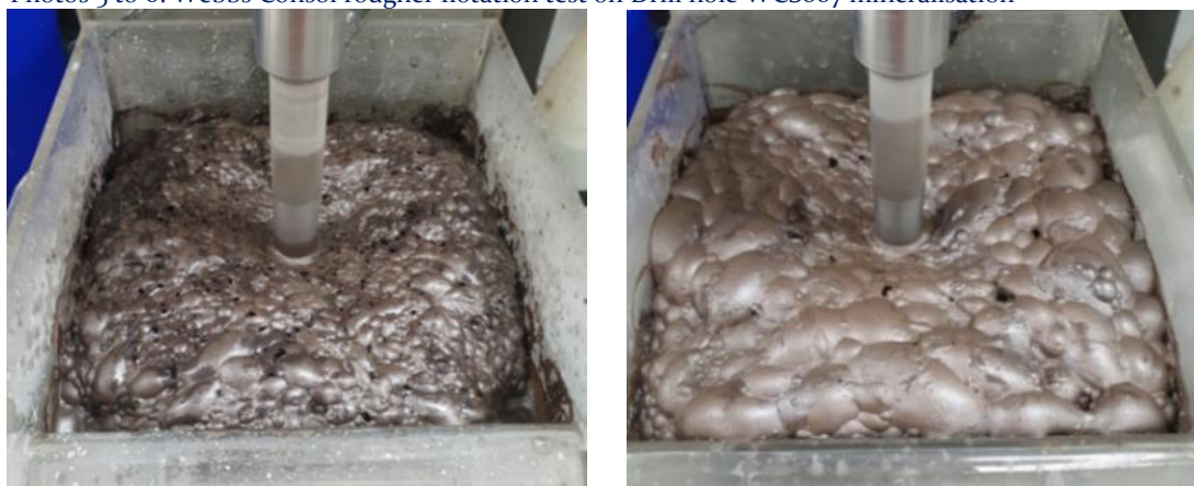
Photos 5 to 6: Webbs Consol rougher flotation test on Drill hole WCS007 mineralisation
