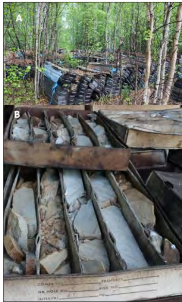
Figure 10-1: Core Storage (A) and Core Trays (B) at Grant site showing muscovite schist (host rock), Felix June 2021.
