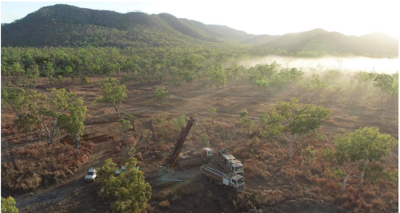
Figure 9: RC rig drilling hole KMRC048 at Orion.
