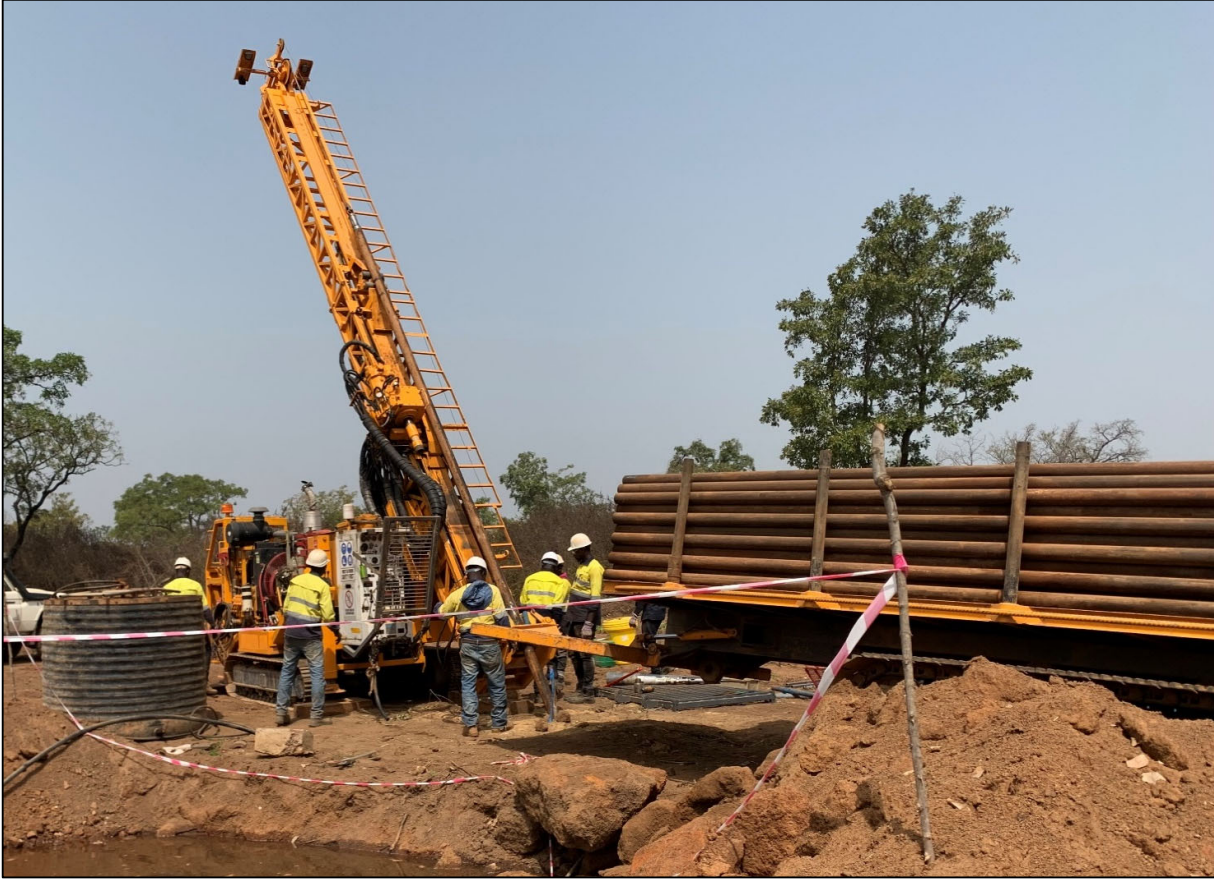
Figure 8: Diamond drill rig (DD) drilling at Tchaga
