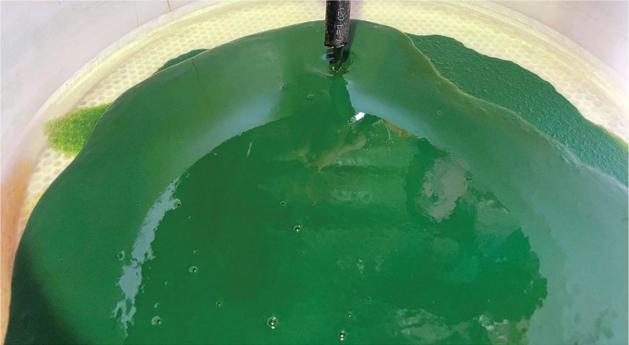
Figure 2 – **Solvent extraction separation of cobalt**
