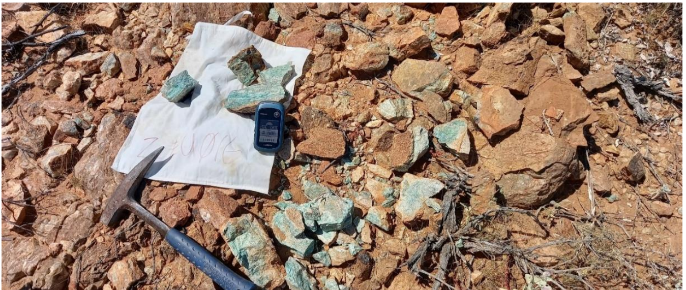
Figure 6. Detail of mineralised outcrop. (Sample# ZEU016 = 1.4% Cu, 0.19% Pb, 125 ppm Zn & 18.4 ppm Ag)
