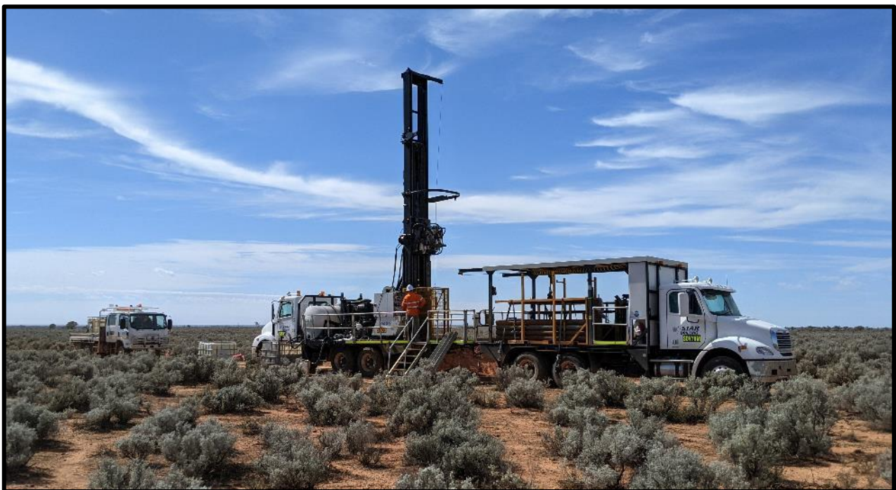
Figure 2 – Sonic core drilling at BBS21-001 Blackbush deposit, Samphire Uranium Project
