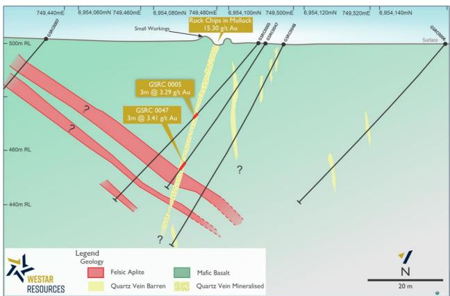
**Figure 3** – Cross-section interpretation from drilling at the historical Tassie's mine area.
