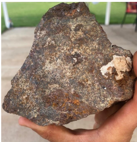
Figure 3: Photo of sample MNRK0529 (39.7% TREO, 6.30% Nd 2 O 3 +Pr 6 O 11 ) showing large reddish brown monazite crystal masses within an ironstone vein from near Y3.
