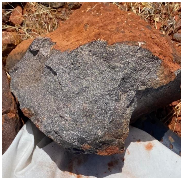
Figure 4: Photo of a niobium vein (MNRK0527 (5.8% Nb 2 O 5 , 0.35% TREO) from near Y3 comprised of quartz, ferrocolumbite, hematite and magnetite.
