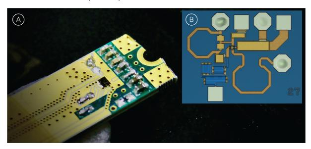
**Image 1.** A The integrated single chip ESR detector based on HEMT. **B** A microscope image of a region in **A** (inside the black square in the centre of the chip) of approximately 0.5mm x 0.5mm showing the miniaturised on-chip ESR componentry used to detect the quantum spin states in Archer's <sup>12</sup>CQ qubit material at room temperature.
