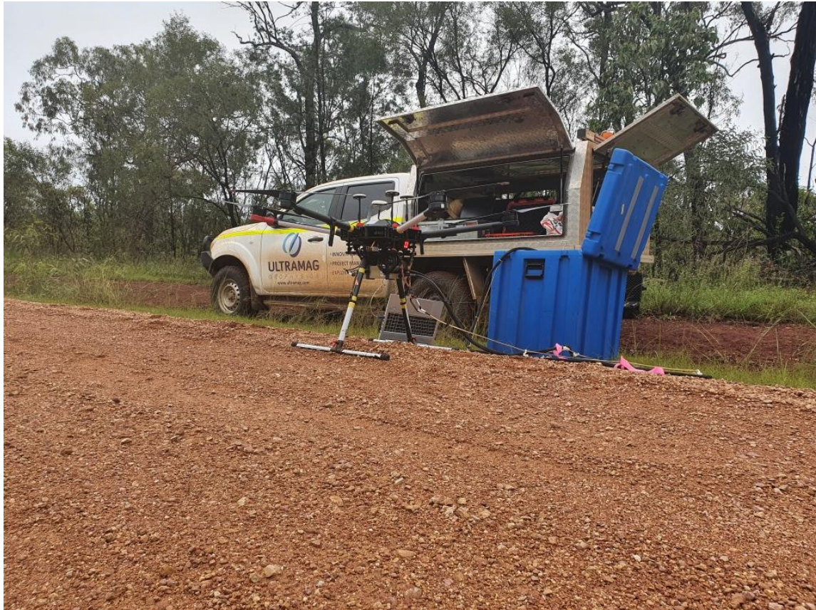
Image 2: UAV being utilised to undertake the drone magnetic survey
