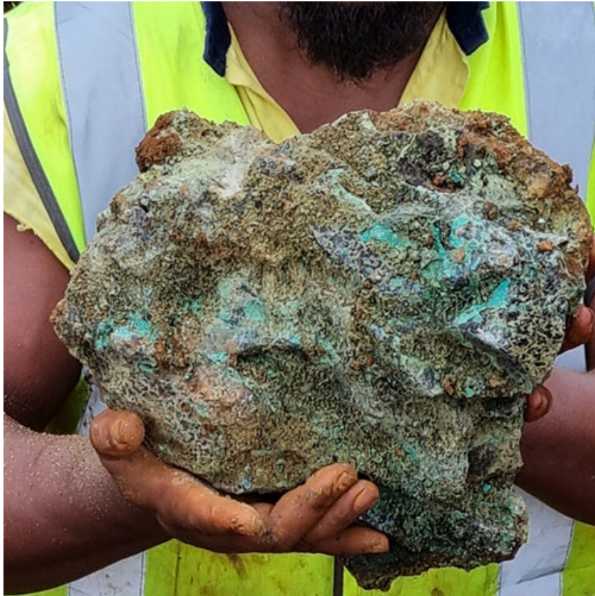
Photo 3. Highly Mineralised Saprolite pod in Test pit. Nickel-bearing material is blue-green in colour.
