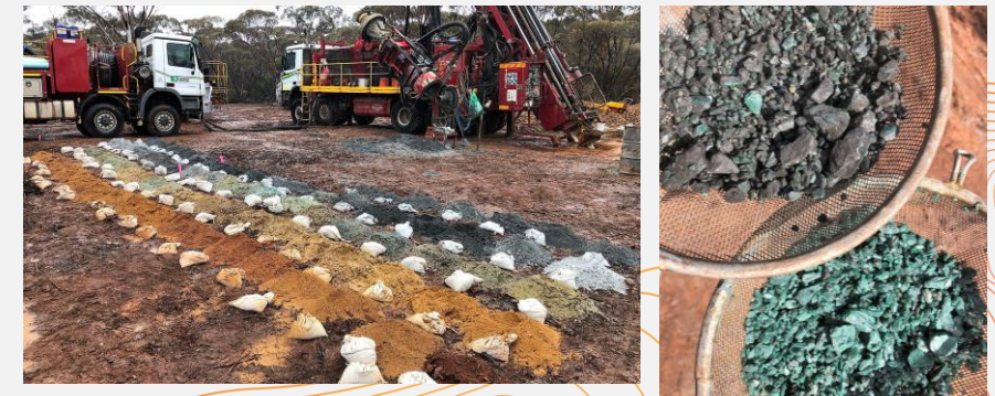
Drill rig at HWRC003 (left) with sieved chips showing contrast between mineralised structure and fuchsite alteration halo (right)
