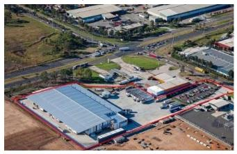
8 Brabham Drive is an A-grade industrial logistics facility designed as a cross-dock incorporating a high clearance, column-free warehouse. Leased to a specialist logistics operator BagTrans, it also features over one hectare of heavy duty, concrete hard stand areas, as well as a truck washing facility.
