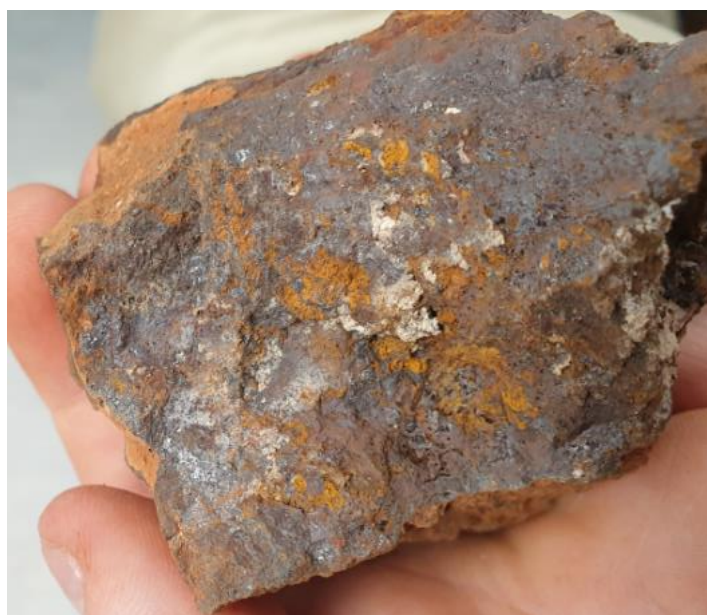
Figure 1: Rock chip sample MNRK0366 from the ~1.2km long northern gossanous horizon showing limonitic staining around boxworks (0.4% Cu, 0.4% Ni, 0.03% Co, 0.3 g/t Pt-Pd-Au).
