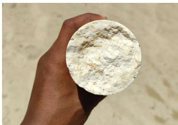
Cross section through Upper Sequence Massive Limestone core - Soalara A3
