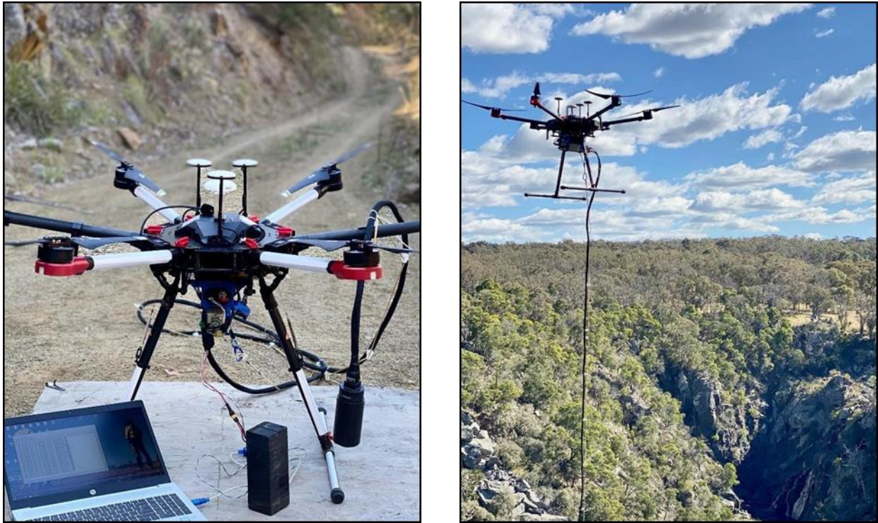
Image 1: UAV's utilised to complete the drone magnetic survey at Gunnawarra
