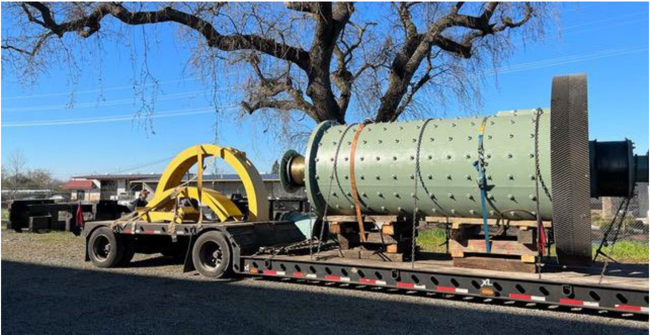
Figure 6: The 250tpd mill loaded for transportation from California to the Lucky Strike mill in Colorado
