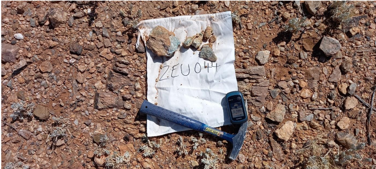
Figure 4. VMS base-metal target; subcropping exhalative malachite, chalcocite, and galena-bearing barite lens. (Sample# ZEU044; 2.19% Cu, 0.2% Pb).
