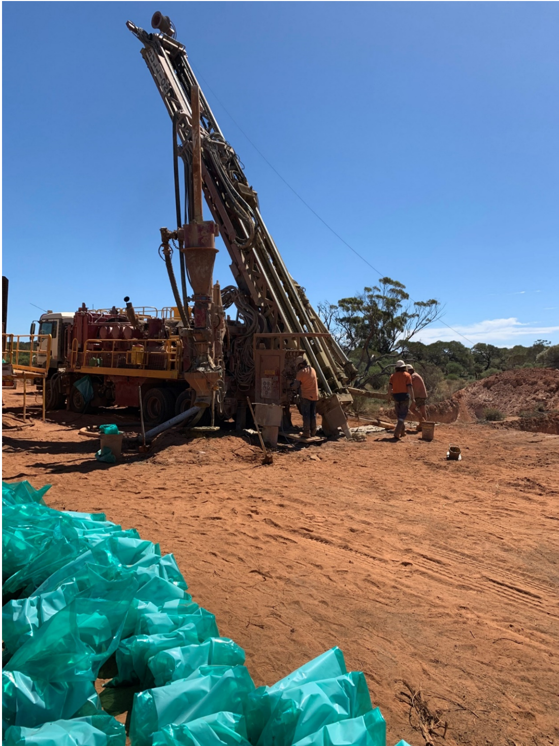
Figure 6: Photo of RC drill rig at Ares with drill chip samples being collected.
