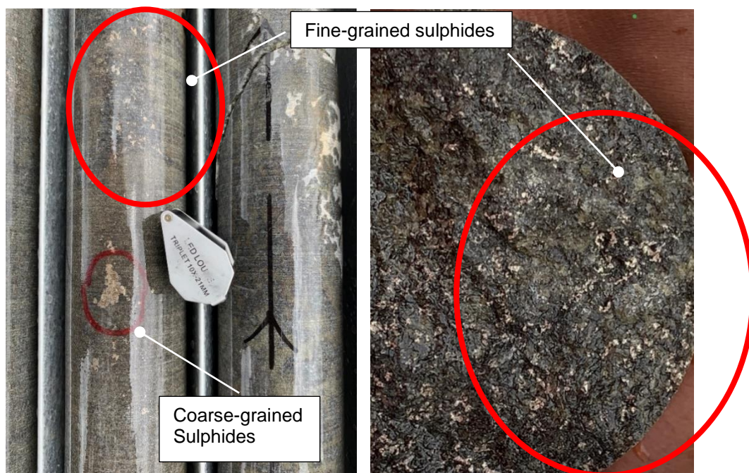
Figure 3 - Disseminated sulphides within the 148 to 161m interval on the broken face of the core and coarser sulphides between 130.2 and 132m shown on the left
