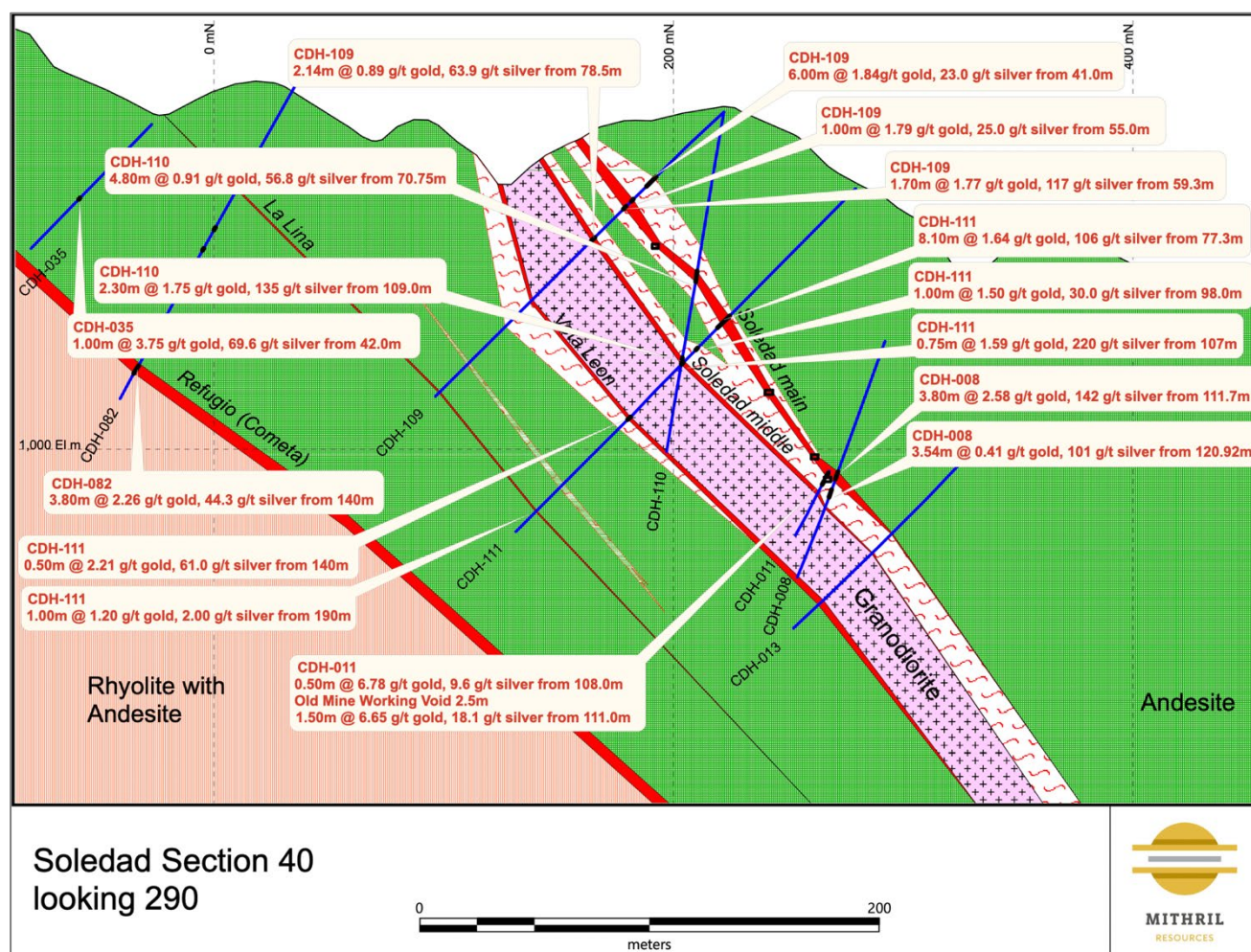
Figure 1 – Cross-section 40 for drill results at La Soledad holes CDH-109 to 111 plus previous drill hole results for holes CDH-008 and 011. Sheeted vein system associated with the granodiorite intrusion.
