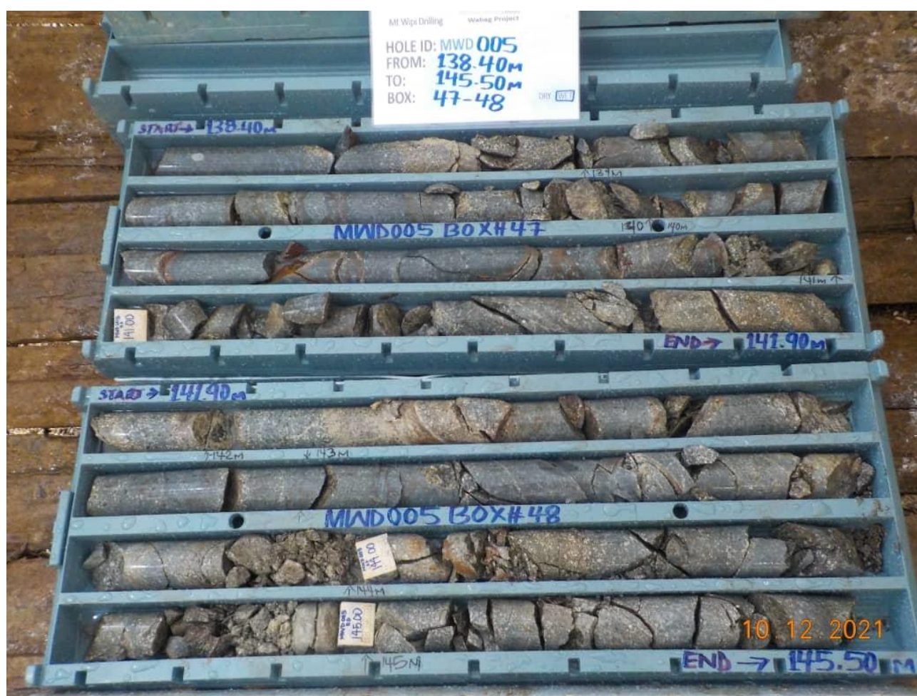
Figure 2. Core from MWD005 where the 11.7g/t gold assay was recorded between 144 to 145m
