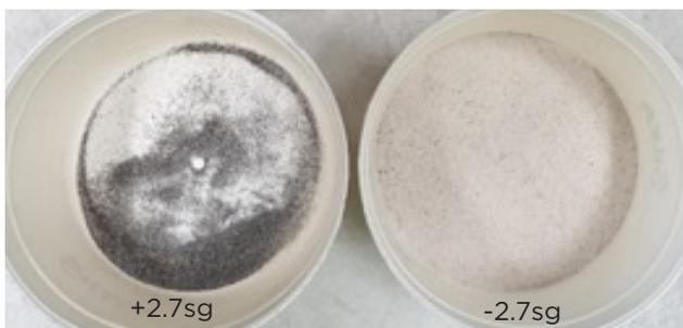
A sub-sample of the float fraction was treated in a high-energy attritioning cell to clean the surfaces of the sand particles. The residence time was five minutes with an operating solids density of ~75%w/w. The attritioned sample was wet-screened at 106µm to remove any liberated slimes. The assay for the attritioned and deslimed product is shown in Table 6.4.
