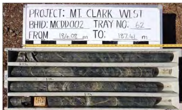
Above: Drill Core Tray from MCDD002 Showing Part of the Interval 14 m at 0.23% Cu (Note the high level stockwork quartz veining and sericite alteration, indicating not yet in core of the system)
