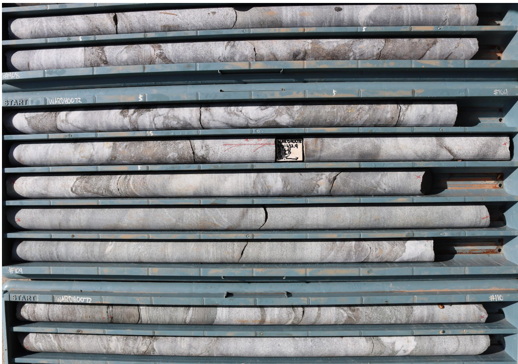
Figure 06: WARDH72 427m- 433m semi-massive pyrrhotite/chalcopyrite sulphide mineralisation
