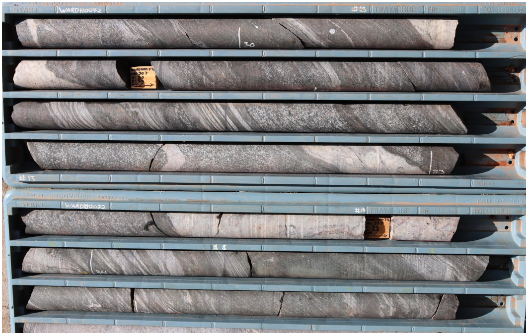
Figure 05: WARDH72 29.5m- 35.5m Intense magnetite +/- copper/base metal sulphide mineralisation
