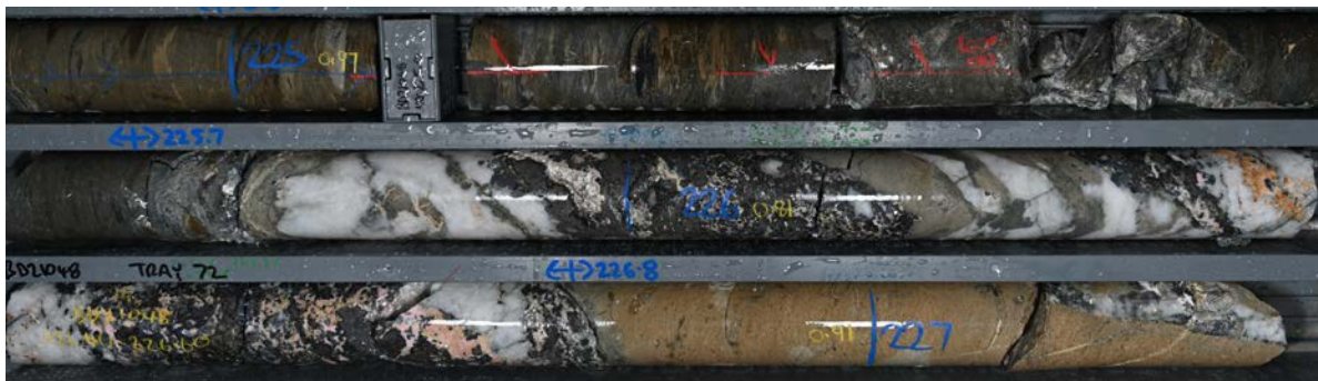
Figure 2. Intercept from BD21048 at 225 metres of quartz-sulphide mineralisation.
