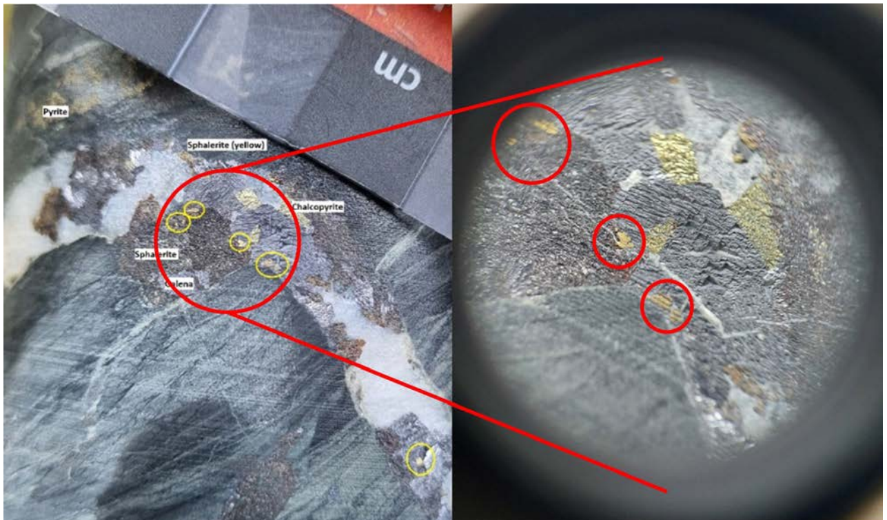
Figure 5. Visible gold. Sheeted calcite-sulphide-gold vein in HQ3 core (left) with a 20x magnification hand lens view (right), 405m in BD22004.
