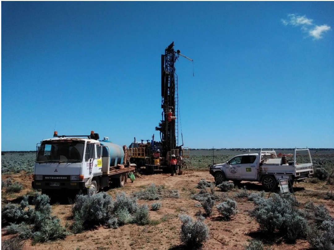
Figure 4: Rotary mud drilling rig at Blackbush deposit, Samphire Uranium Project
