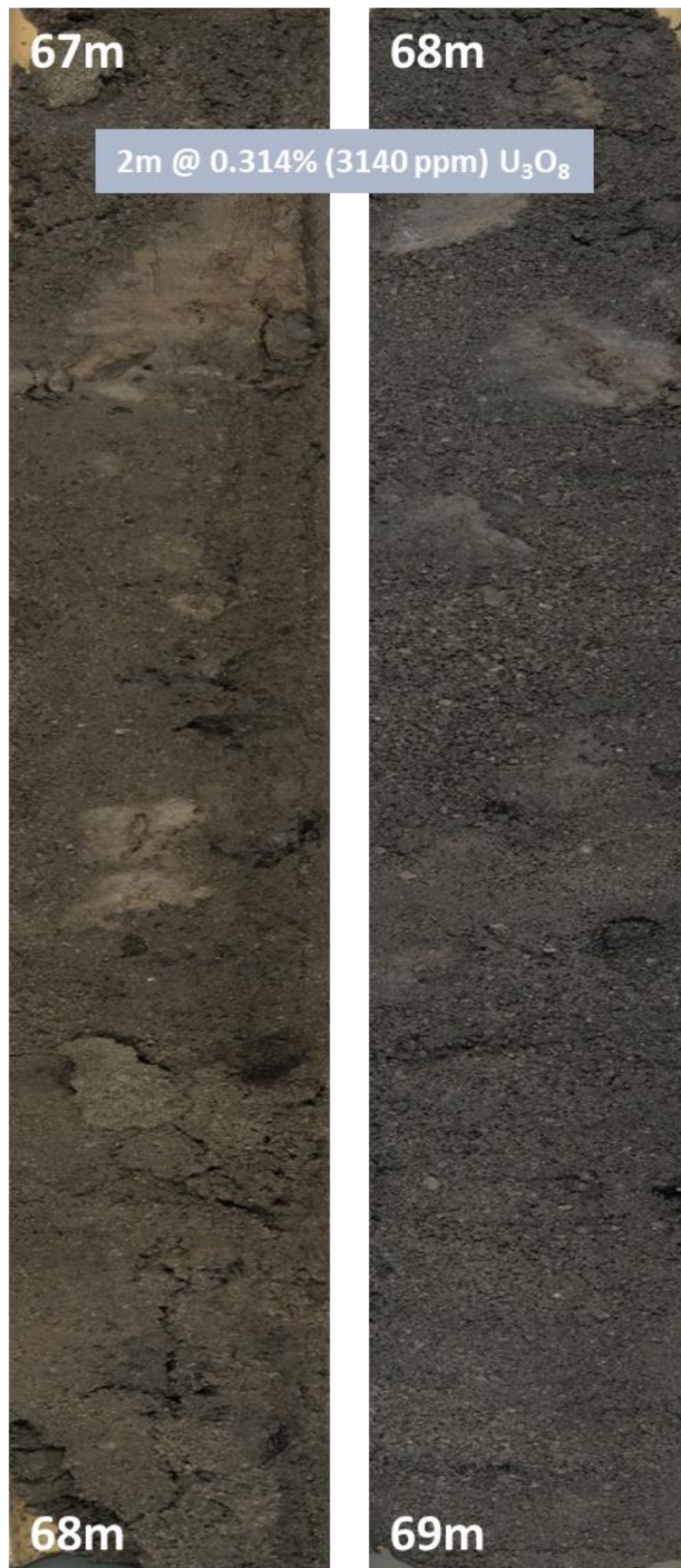
Figure 3: Example of mineralised permeable lithologies (Kanaka Beds) observed in sonic core hole BBS21-002, depth 67m-69m (U 3 O 8 ppm reported from assay).
