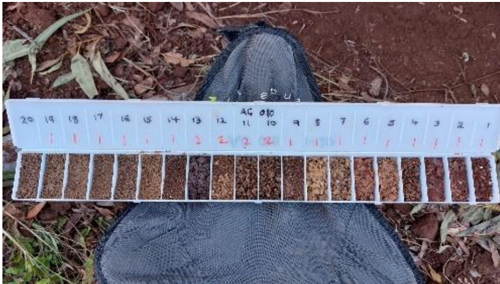
Images 3-6: Chip trays from reverse circulation hole #10 showing 1m intervals from surface
