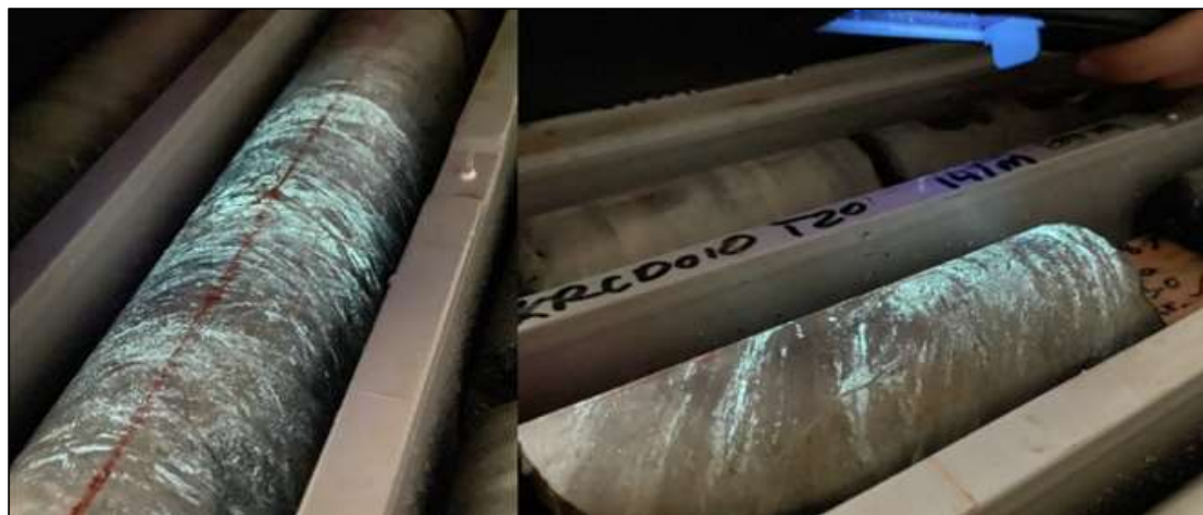
Bornite (copper sulphide) with malayaite (calcium-tin-silicate) fluorescing under UV light in 3KRC0010. Drillcore is 61.1mm wide for scale.
