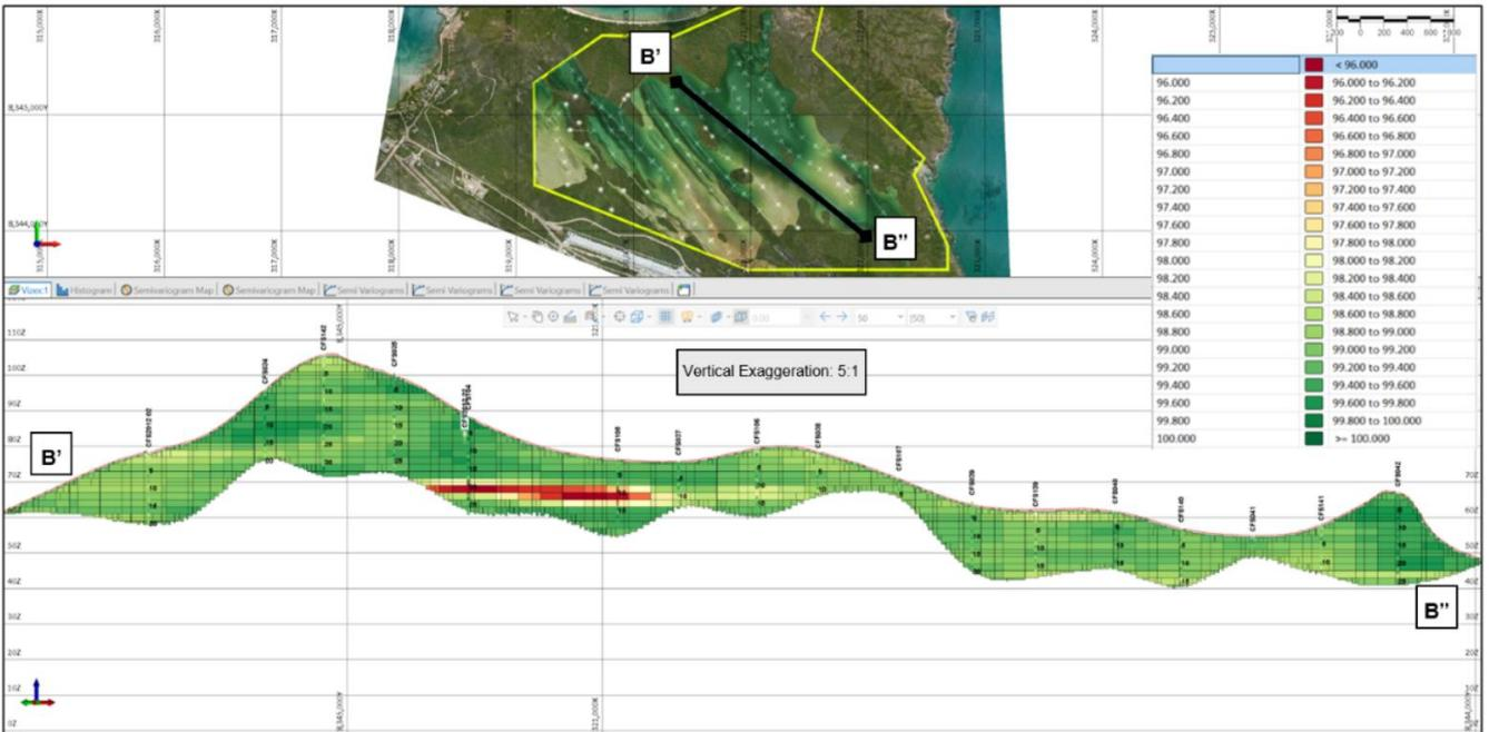
Figure 3: Cape Flattery Silica Project – typical deposit long section
