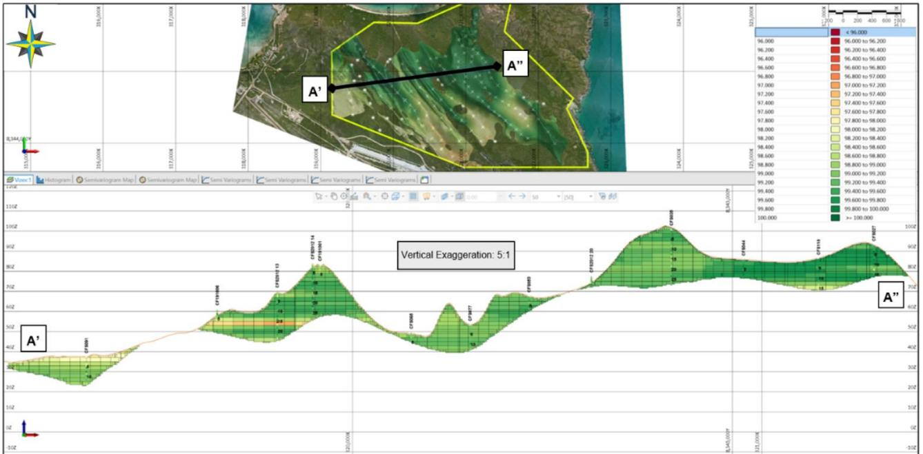
Figure 2: Cape Flattery Silica Project – typical deposit cross section
