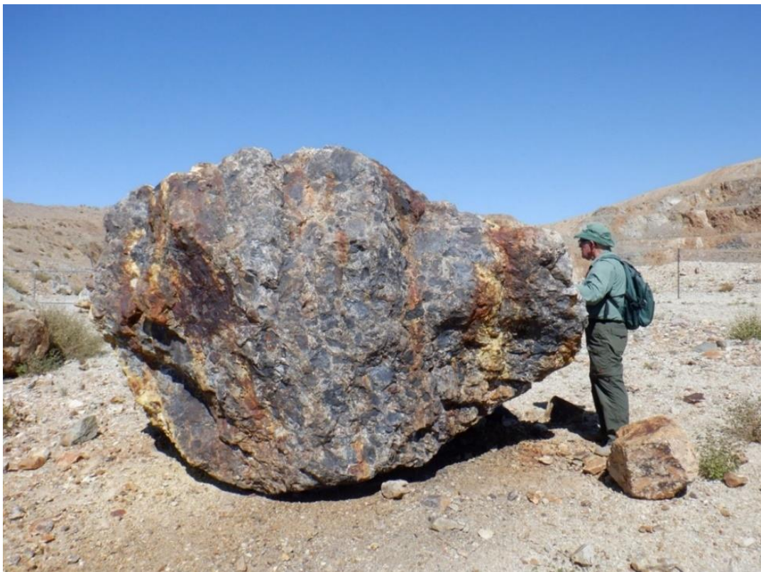
Figure 5. Breccia waste rock at south rim of Colosseum mine pit where sample COR-1 was collected. Photo (a) shows radiometric reading ( \mu\text{R/h} ) of the rock sampled. Photo (b) Dr Anthony N. Mariano, PhD studying the nature of the breccia waste rock.
