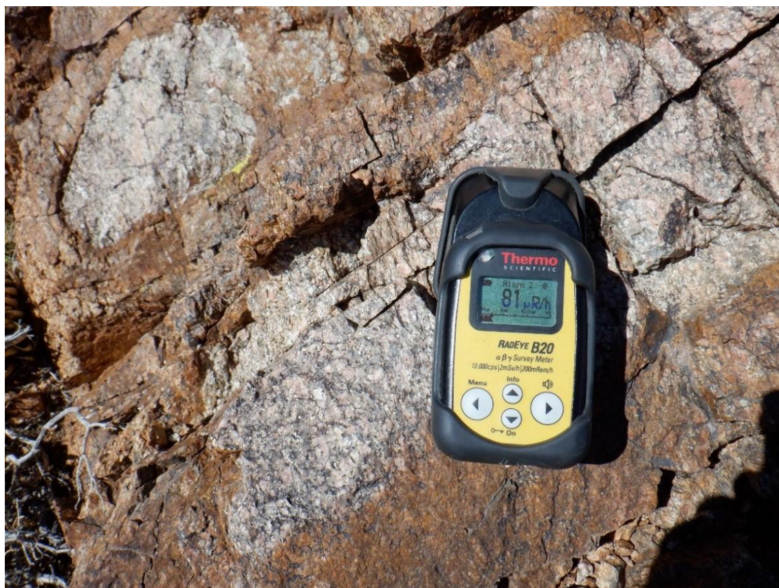
Figure 8. Outcrop on the ridge at the southern extent of the Colosseum mine property where sample COR-4 was collected (a). Photo (b) radiometric reading ( \mu\text{R/h} ) of the rock sampled.
