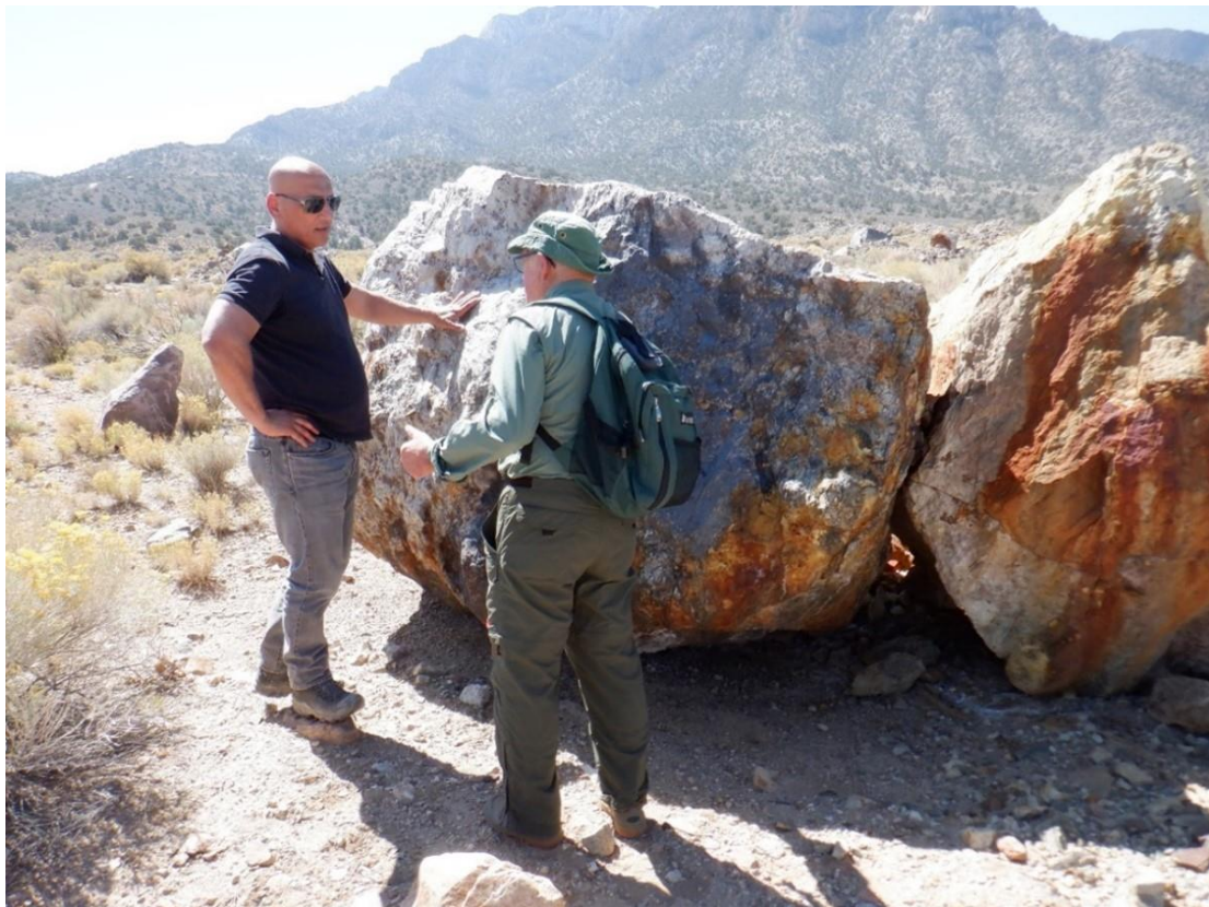
Figure 6. Breccia waste rock in Colosseum mine tailings area where sample COR-2 was collected. Photo (a) shows radiometric reading ( \mu\text{R/h} ) of the rock sampled. Photo (b) The waste rock that Dr Anthony N. Mariano, PhD collected sample COR-2 from
