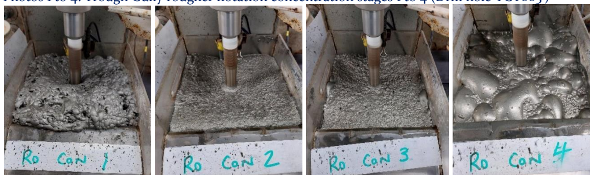
Photos 1 to 4: Trough Gully rougher flotation concentration stages 1 to 4 (Drill hole TGY003 1 )
