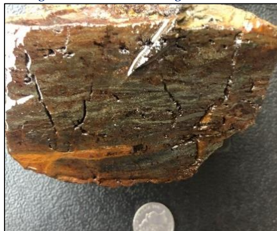
Photo 6: Trough Gully Mine foliated sulphide veining – evidence of boudinage structures
