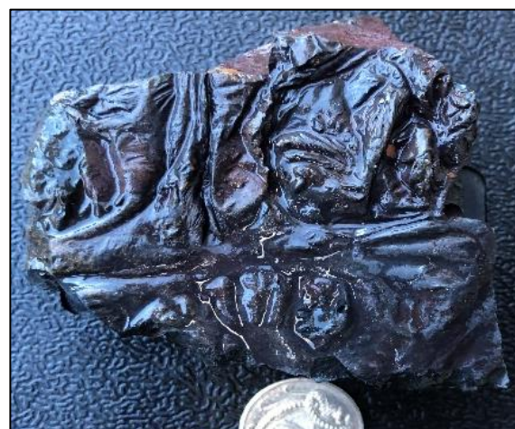
Photo 5: Trough Gully historical smelter slag
